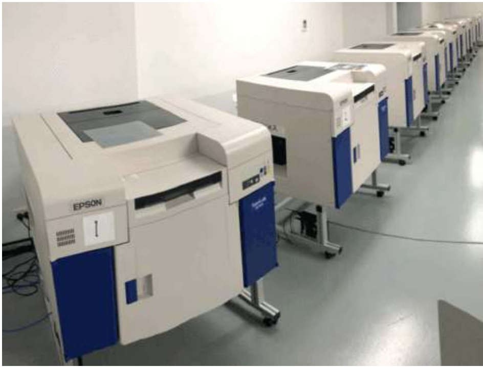
Epson Surelab D3000 inkjet 'drylabs' daisy-chained to create a high volume photo printing installation.
